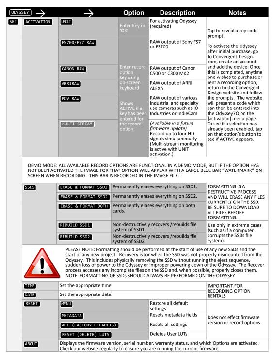
The remainder of the menu replicates controls available on the Upper Tool Bar when the Odyssey is in RECORD mode.
